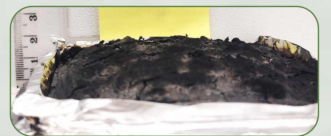
Bio-PUD coating with fire retardant (Bio+FR_1) during and after cone calorimeter test.
