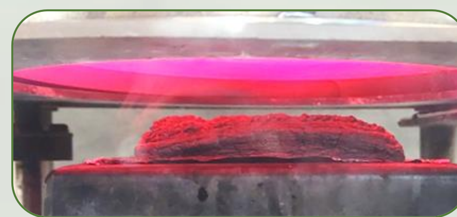
Bio-PUD coating with fire retardant (Bio+FR_1) during and after cone calorimeter test.
