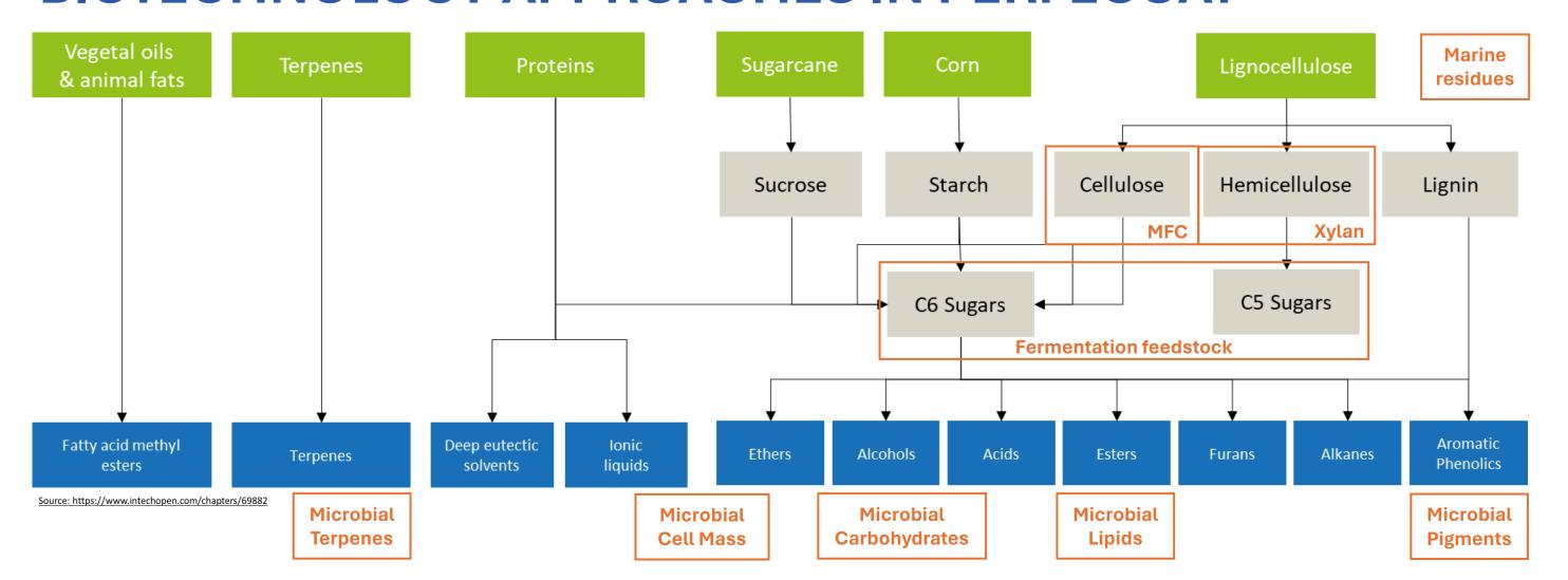
The PERFECOAT project applies biotechnology to produce microbial polymers, lipids, terpenes, pigments, and cell mass from biomass sugars, as well as biopolymers through chemoenzymatic extraction from lignocellulose and marine residues. Chemical upgrading of these base compounds, guided by rigorous testing provides the required physical and chemical properties and activation for use as bio-based ingredients in new paint formulations with desired performances.
