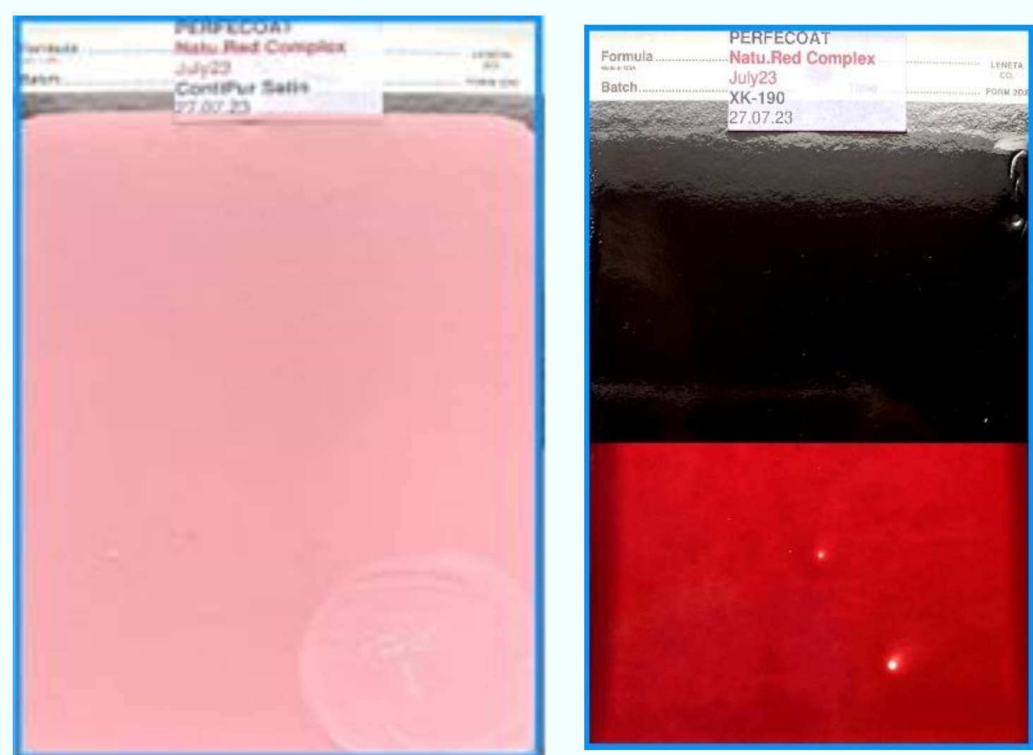
Natu.Red Complex – a novel natural red pigment here tested in a white base paint, and in a clear coat.
